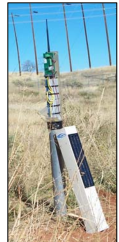
Model FGRCP LineMarker Test Station on 3 inch conduit pipe.
